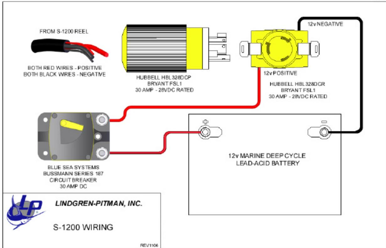
Power Requirement and Wiring: 12-volts DC Max 30Amps
